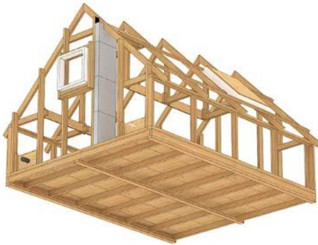
Figure 5. Bottom view of floor structure. Width 3220 mm. Length: 4000 mm.
