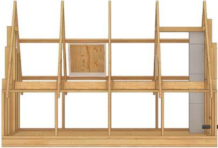
Figure 1. Front view 4 m. Roof surface without skylight. Collar tie in rafters 2 and 3 from the left cut off, in order to fit a vapour control layer to the ridge here. 900 mm from bottom of sole plate to top of wall plate in wall.
