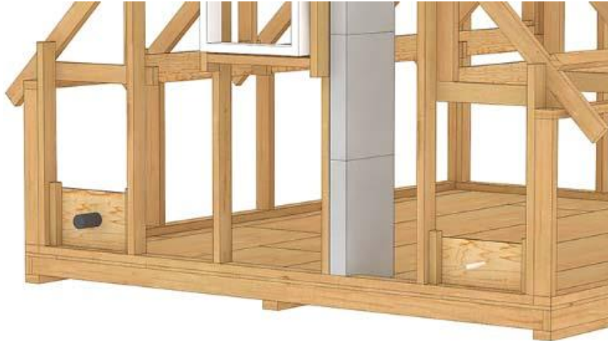
Figure 7. Solid support around penetration points for PP-pipes Ø 75 mm (left) and power cable (right) respectively. The gable window is placed in a clearance, made using 95 mm battens.
