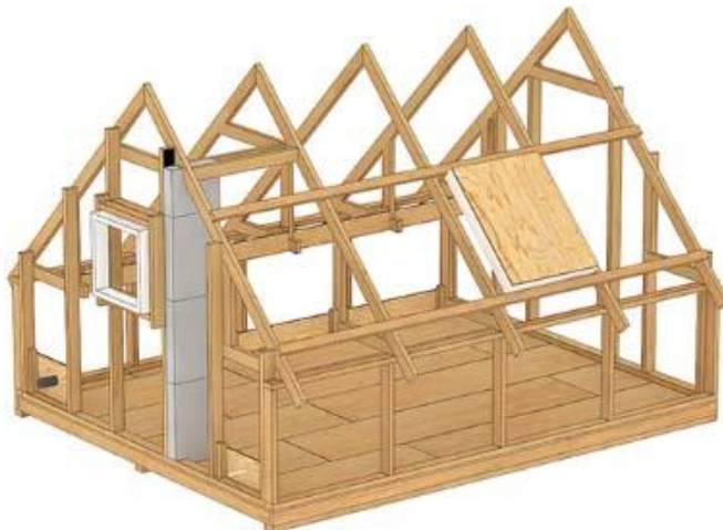
Figure 6. The 2 rear collar ties are cut off, in order to take the vapour control layer to the ridge. Joints between floor plates to be sealed, e.g. using vapour control layer tape and membrane as necessary. The gable window is placed in a clearance, made using 95 mm battens.
