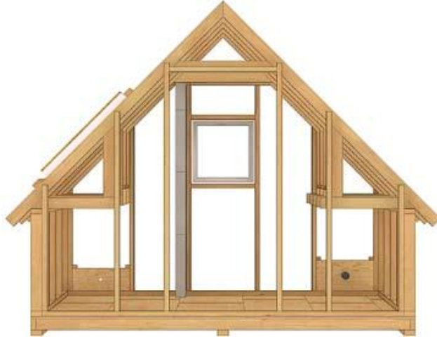
Figure 4. Gable with 900 x 2000 mm rough opening, where the equipment for measurement of air permeability of buildings may be fitted. Beam ends on left cut flush with knee wall: 700 mm from inner side of knee wall to outer side of outer wall.
